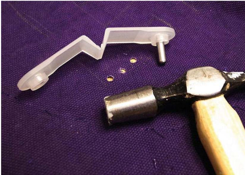
**Figure 6-11.** *Punching holes for the eyelets*
