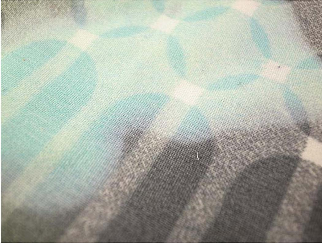
*Figure 4-2. Thermochromic screen print after heat is applied*
