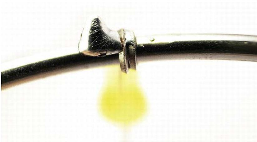
**Figure 5-23.** *A cold soldering joint*
