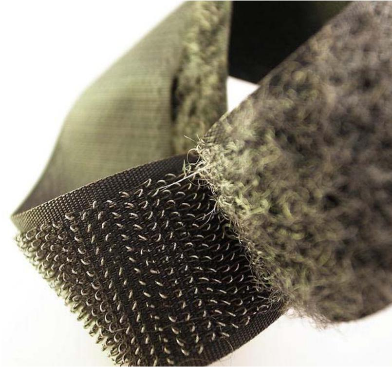
**Figure 4-7.** *Conductive Velcro*
