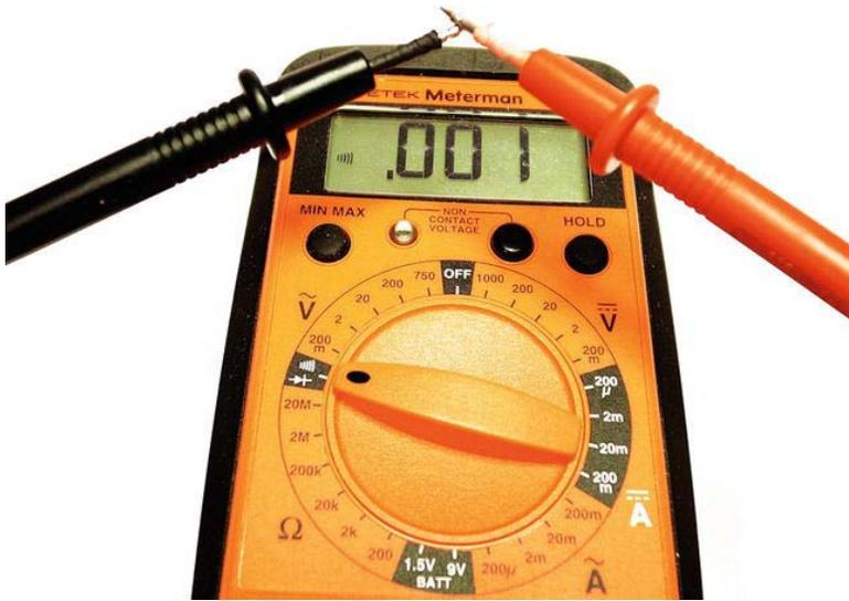
**Figure 5-1.** Finding conductivity with a multimeter
