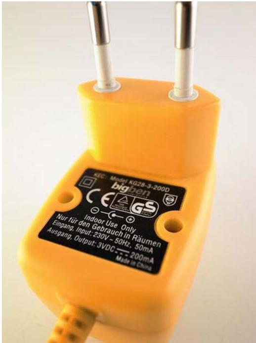
**Figure 3-13.** Transformer supporting a 230V input and a 3V output
