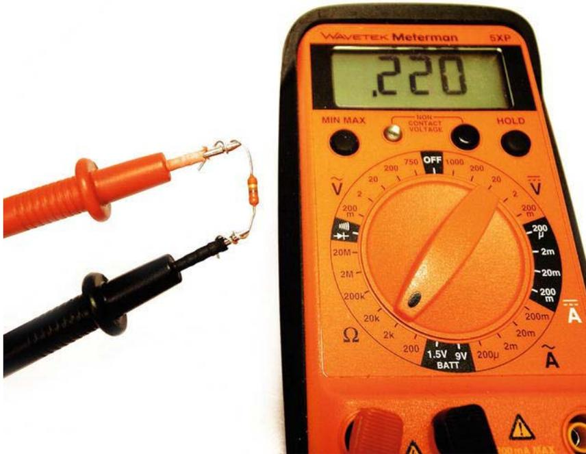
**Figure 5-3.** *Measuring the resistance of a resistor*
