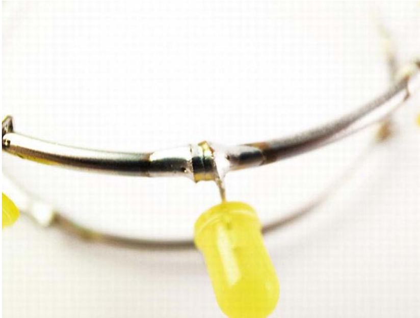
**Figure 5-24.** *The solder should spread onto the material.*
