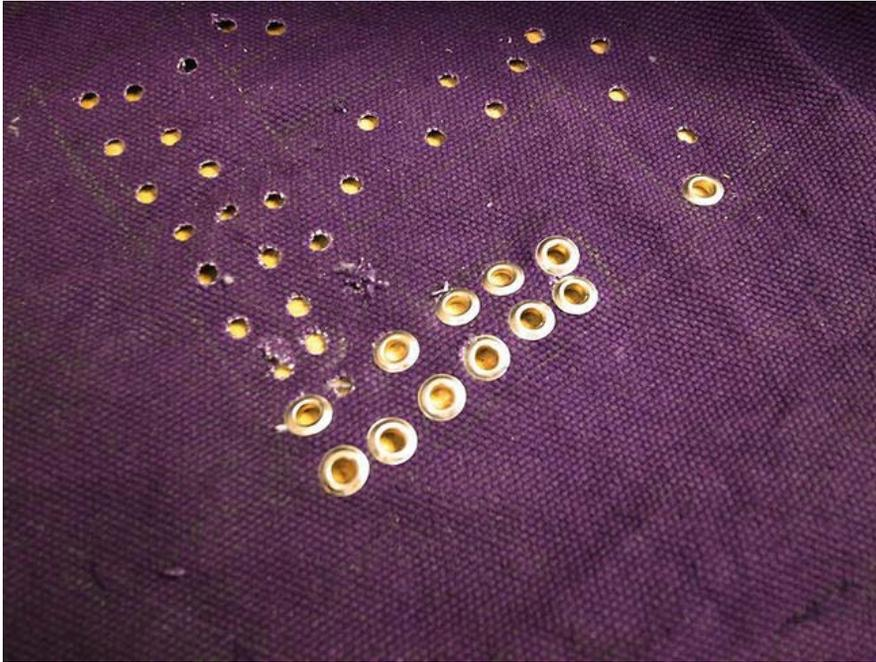
*Figure 6-12. Eyelets punched in place*
