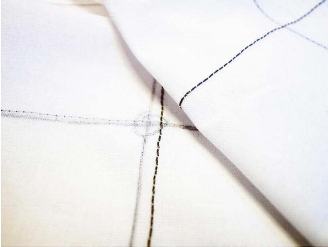
**Figure 11-5.** *Conductive thread matrix*
