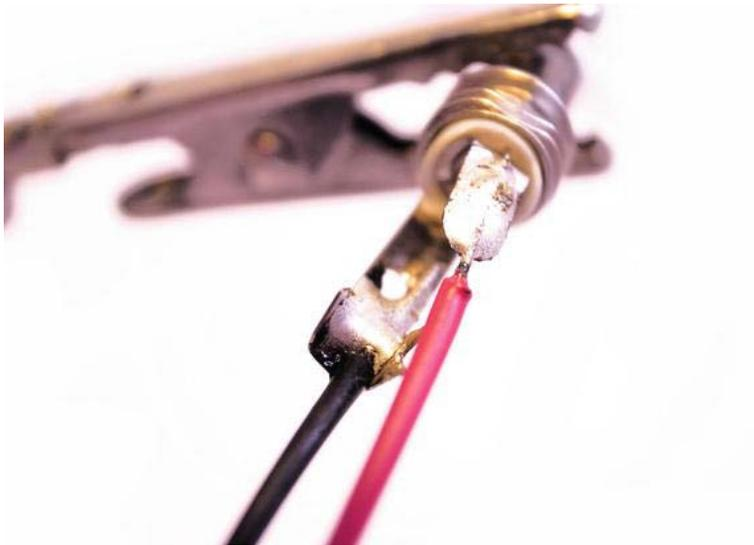
**Figure 13-19.** Soldering the DC connector
