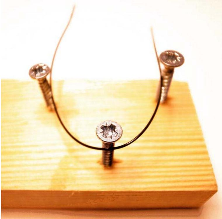
**Figure 12-12.** *Reprogramming the SMA wire*
