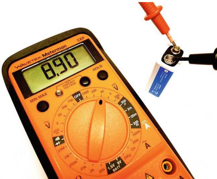
**Figure 5-4.** *Measuring voltage*
