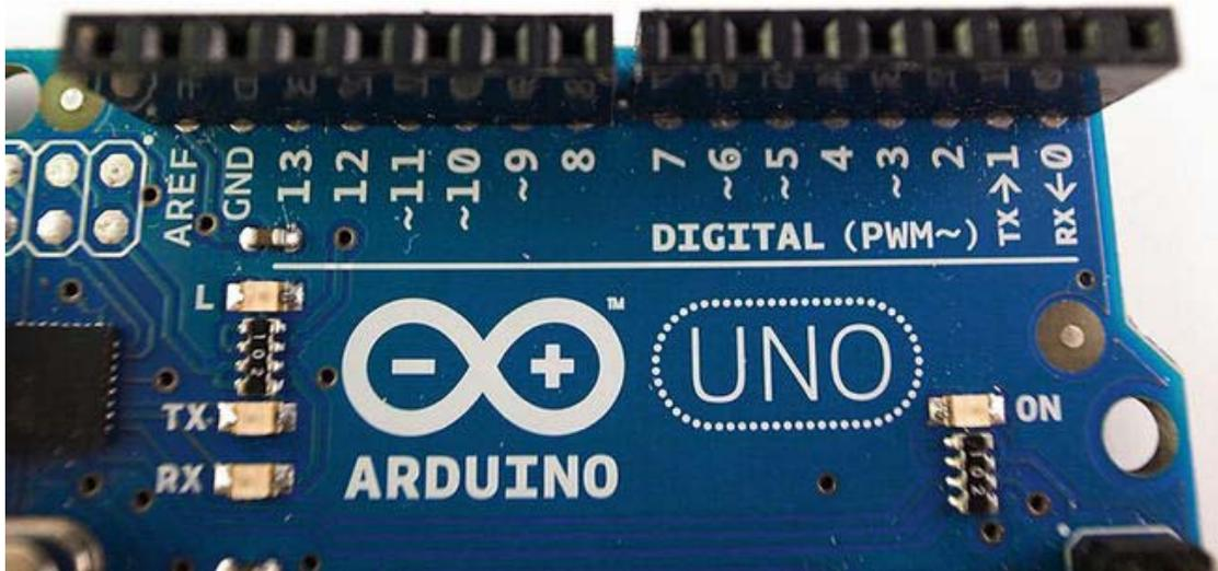
**Figure 3-9.** Digital pins from 0 to 13
