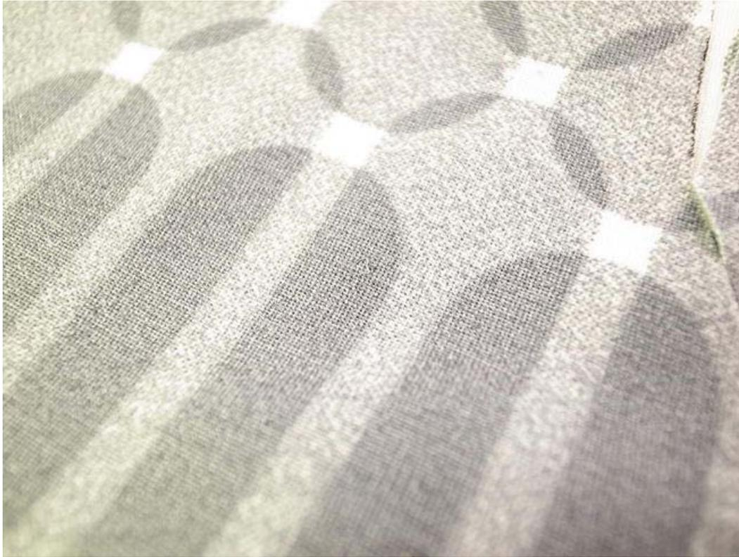
**Figure 4-1.** Thermochromic screen print on fabric
