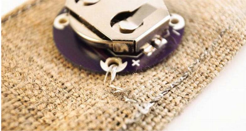
**Figure 5-16.** Making the power connection
