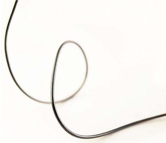
**Figure 4-9.** Smart wire that remembers shapes
