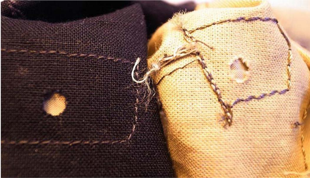
*Figure 7-7. Conductive thread connections*
