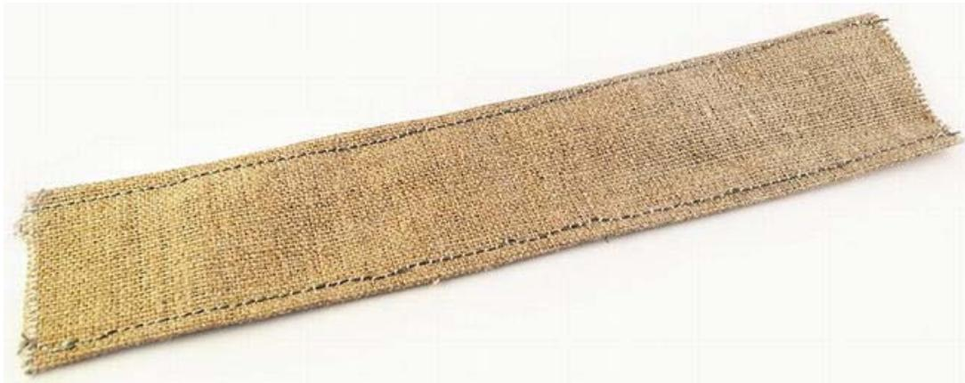
**Figure 5-12.** Seams sewn with conductive thread
