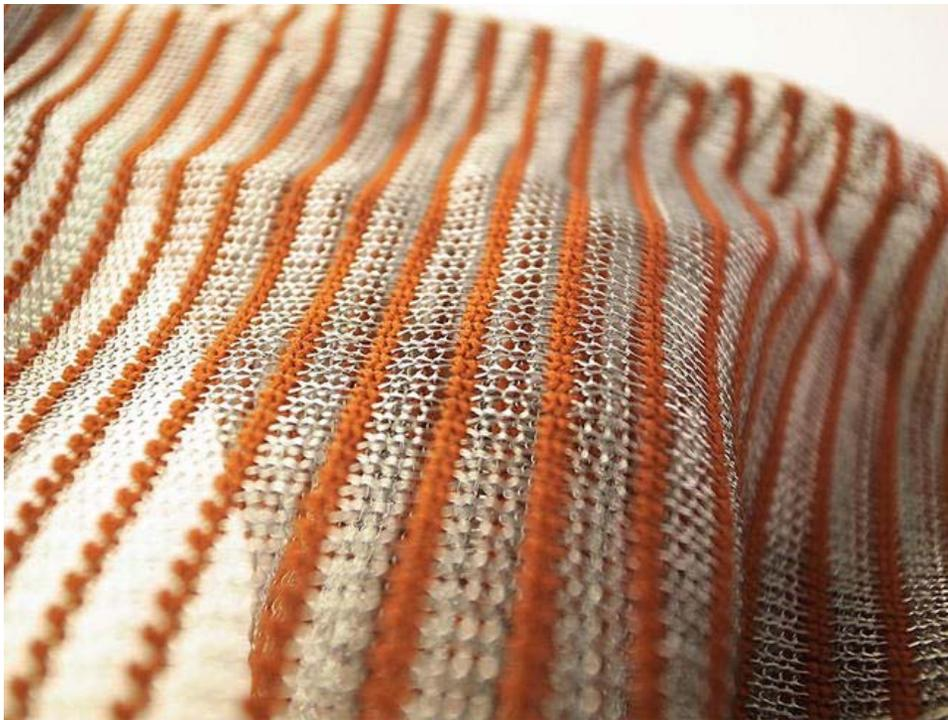
**Figure 4-6.** Conductive mesh fabric mixed with non-conductive thread
