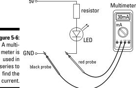
Figure 5-6: A multiused in series to find the current.
