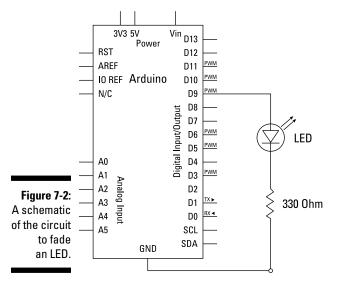
After you assemble your circuit, you need the appropriate software to use it. From the Arduino menu, choose File⇔Examples⇔01.Basics⇔Fade to call up the Fade sketch. The complete code for the Fade sketch is as follows:
