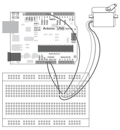
Figure 8-9: A servo motor wired to your Arduino.
