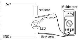
A good way to test your multimeter is to measure the voltage between the 5V pin and GND on your Arduino. Make sure that your Arduino is plugged in, and connect a jump wire to each pin to make them easier to access with your probes. Place the red voltage probe on the 5V wire and the black common probe on the GND wire. This should return a value of 5V on the screen of your multimeter and prove that your Arduino is supplying 5 volts as expected.
