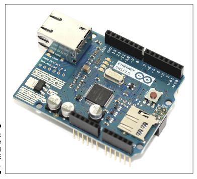
Figure 13-7: An Ethernet Shield (without PoE module).
