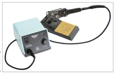
Figure 10-4: A Weller solder station.
