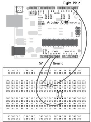
Figure 7-8: Pin 2 is reading the pushbutton.
