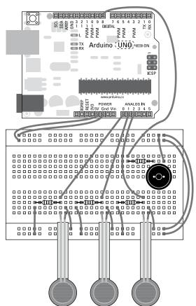
Figure 12-5: A button circuit layout.
