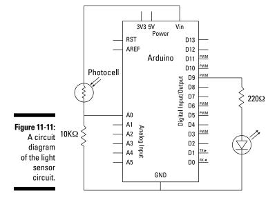
Build the circuit and go to File Examples 33. Analog Calibration and to find the sketch. The code for this example is as follows:
