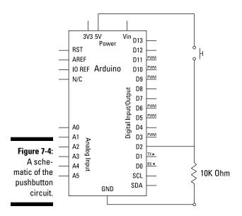
Build the circuit and upload the code from File Examples 202. Digital Button.
