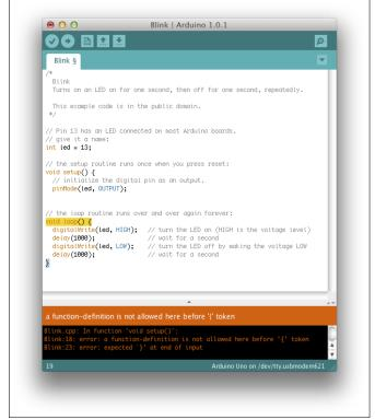
Figure 4-10: The Arduino software is telling you that a bracket is missing.
