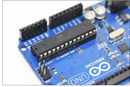
Figure 4-4: Close-up of the ATmega-328P-PU chip.
