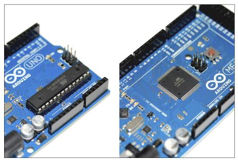
Figure 14-2: PDIP and TQFP.
