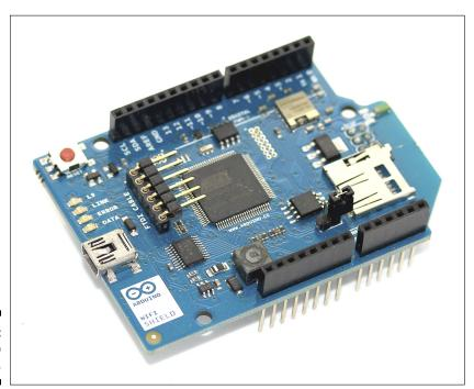
Figure 13-8: The Arduino WiFi Shield.
