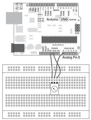
Figure 7-6: The potentiometer is connected to Analog Pin 0.
