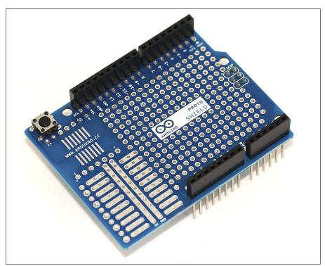
Figure 13-1: A fully assembled Proto Shield.
