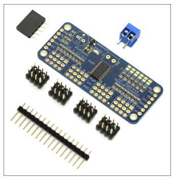
Figure 15-1: I<sup>2</sup>C PWM/ Servo Driver board.
