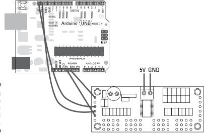
Figure 15-4: Diagram of a PWM Driver board wiring.
