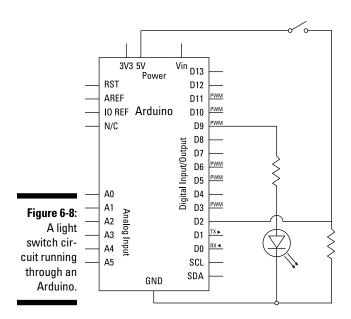
The large, caterpillar-shaped item on the diagram is the Arduino. This is the standard symbol for an integrated circuit and is similar to the physical representation — a rectangle with lots of legs poking out. All the legs or pins are labeled so that you can tell them apart.
