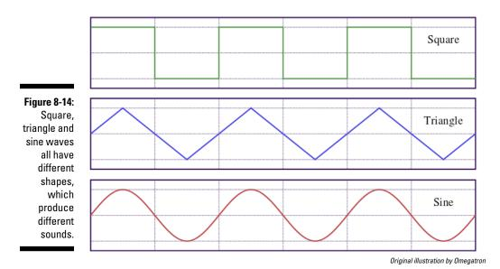
Digital devices like this as well as other electronic instruments generate square waves, resulting in a buzzing sound. The buzzer isn't restricted to just one pitch. By changing the frequency that the buzzer is switched at (the width between the square waves), you can generate different frequencies and therefore different notes.
