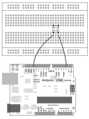
Figure 12-1: The pushbutton circuit layout.
