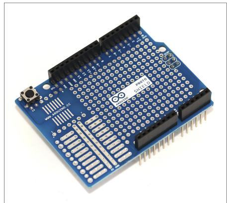
Figure 10-12: A complete Proto Shield.
