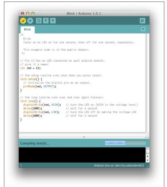
Figure 4-8: The progress bar shows that the sketch is compiling.
