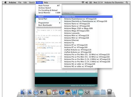
Figure 4-5: Select Arduino Uno from the Board menu.
