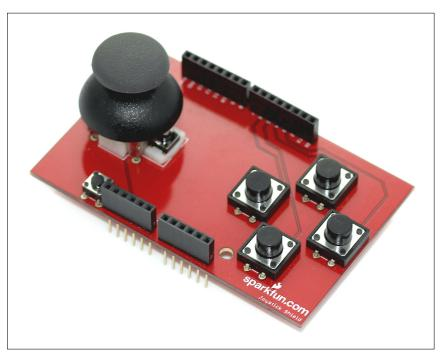
Figure 13-4: A Joystick Shield.
