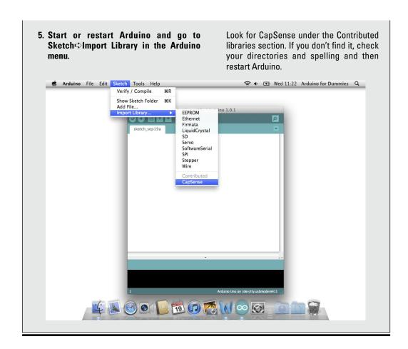
The easiest way to make a capacitive sensor is to use the CapSense library by Paul Badger. By using the CapSense library (I explain how in the "Getting the CapSense Library" sidebar), you can do away with mechanical switches altogether and replace them with highly robust capacitive touch sensors or capacitive presence detectors.
