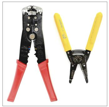
Figure 10-8: Manual and mechanical wire strippers.
