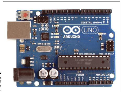
Figure 2-1: The front of an Arduino Uno R3.
