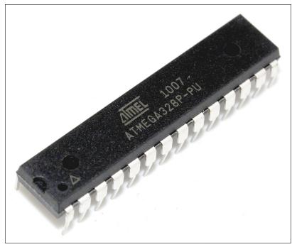
Figure 2-3: An ATmega328 microcontroller all by itself.
