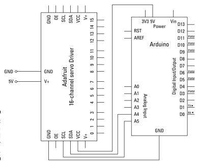
Figure 15-5: A schematic of a PWM Driver board.
