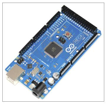
Figure 14-1: An Arduino Mega 2560.
