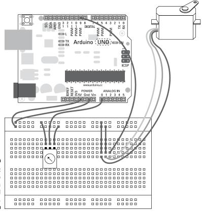
Figure 8-11: A servo motor with control knob.
