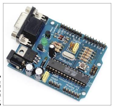
Figure 1-3: The original Arduino Serial board.
