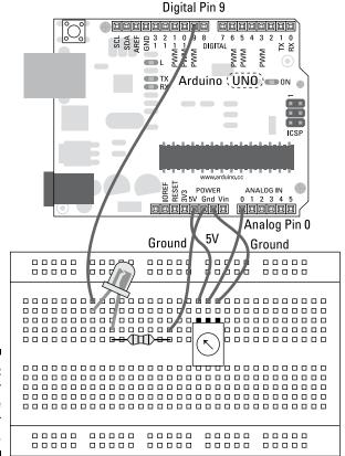
Figure 7-11: Dimmer circuit to be read over serial.
