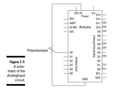
Build the circuit and upload the code from File⇔Examples⇔03.Analog⇔ AnalogInput.
