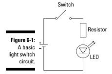
In this circuit, you have a source of electrical power in the form of a battery. Power is supplied in watts and is made up of voltage (in volts) and current (in amps). Voltage and current are supplied to the circuit through the positive (+) end of the battery.
