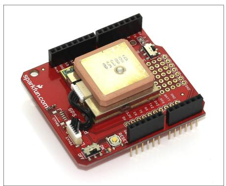
Figure 13-6: The Sparkfun **GPS Shield** with the EM-406a.
