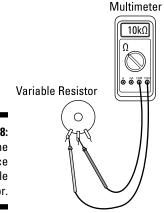
Figure 5-8: Finding the resistance of a variable resistor.
