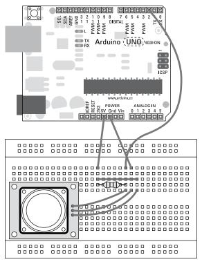
**Figure 12-11:** A PIR sensor circuit layout.
