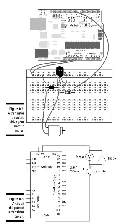
Build the circuit as shown, and open a new Arduino sketch. Choose the Save button and save the sketch with a memorable name, such as myMotor, and then type the following code:
