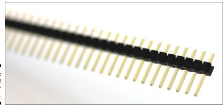
Figure 10-14: Close up of the header pins.
