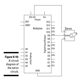
Complete the circuit as described and open the Sweep sketch by choosing File\$\times\text{Examples}\$ Servo\$\times\text{Sweep}. The Sweep sketch is as follows:
