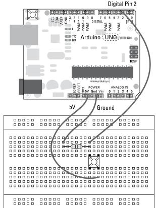
Figure 7-3: Pin 2 is reading the pushbutton. From the schematic in Figure 7-4, you can see that the resistor leading to ground should be connected to the same side as pin 2, and that when the button is pressed, it connects those to the 5V pin. This setup is used to compare ground (0V) to a voltage (5V) so that you can tell whether the switch is open or closed.
