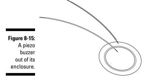
Connect the piezo buzzer to the breadboard and use a set of jump wires to connect it to digital pin 8 on one side and ground on the other. Some piezos have a polarity, so make sure that you connect the positive (+) to pin 9 and the negative (-) to GND. Other piezos don't have a polarity, so if you see no symbols, don't worry. The piezo circuit is shown in Figure 8-16, and the circuit diagram appears in 8-17.
