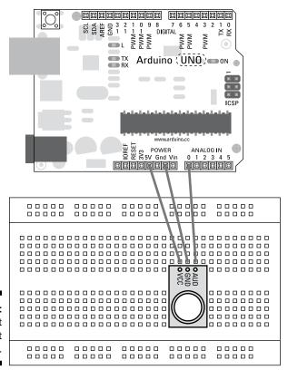
Figure 12-15: An electret mic circuit layout.
