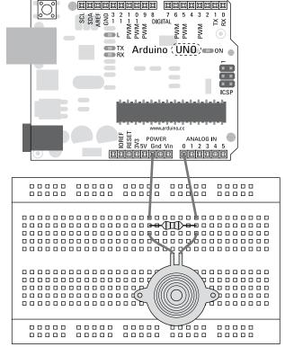
Figure 12-3: A knock sensor circuit layout.
