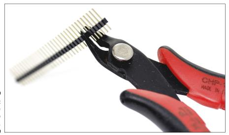
Figure 15-2: Cutting the headers to length.
