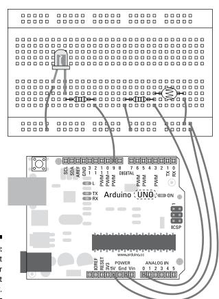
Figure 11-10: The light sensor circuit layout.
