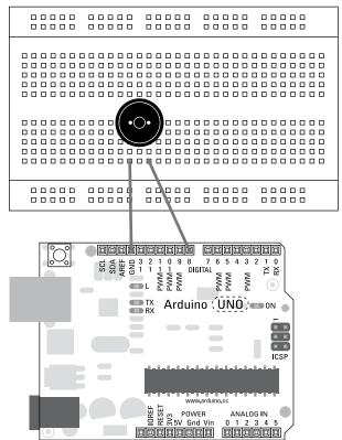
Figure 8-16: A piezo buzzer circuit.
