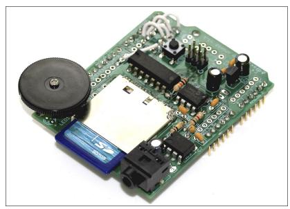
A fully assembled Wave Shield.
