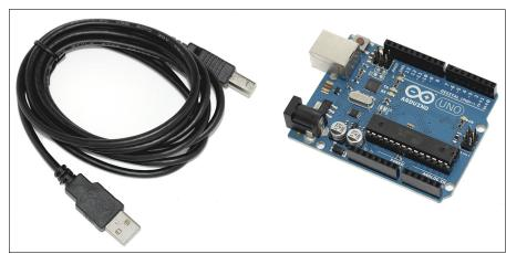
Figure 3-1: An A-B USB cable and Arduino Uno.
