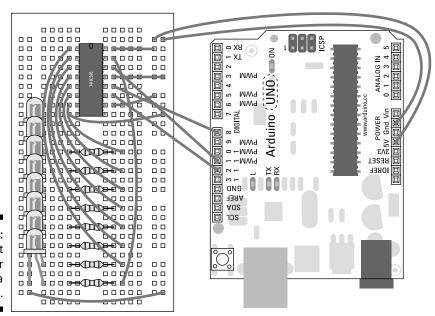
A circuit layout for using a 74HC595.
