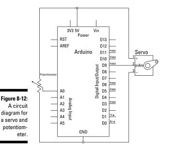
After you have built the circuit, open the sketch by choosing File⇔Examples⇔ Servo⇔Knob. The code for the sketch is as follows:
