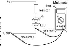
Figure 5-9: Checking the continuity of your circuit.
