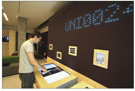
Figure 9-5: The hidden LED display lights up from underneath the wallpaper.
