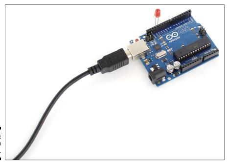
Figure 4-12: Arduino LED Pin 13.
