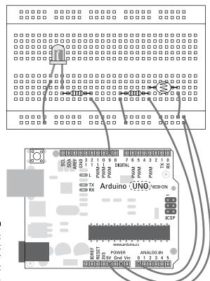
Figure 11-8: The light sensor circuit layout.
