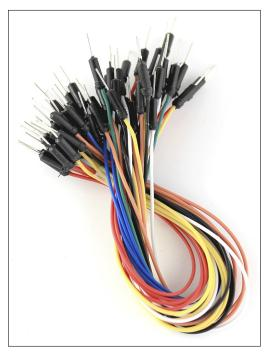
Figure 5-2: A selection of jump wires.
