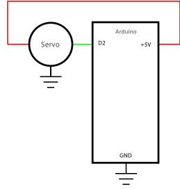
Figure 4-5. Arduino/servo schematic
