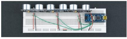
Figure 5-10. The three ultrasonic sensors connected
