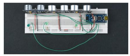
Figure 5-12. LEDs connected for testing
