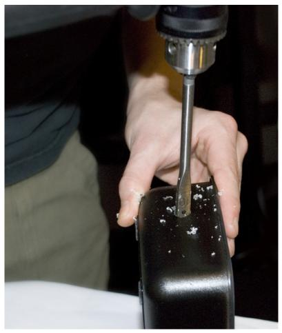
Figure 7-33. Drilling a hole for the USB cable
