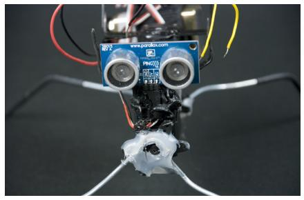
Figure 4-24. Ultrasonic sensor in place
