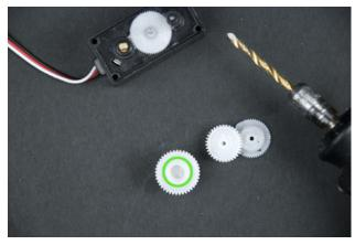
Figure 8-14. Rounding out the dent in the gear
