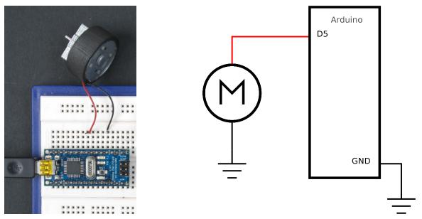
Figure 3-15. Connecting a vibration motor
