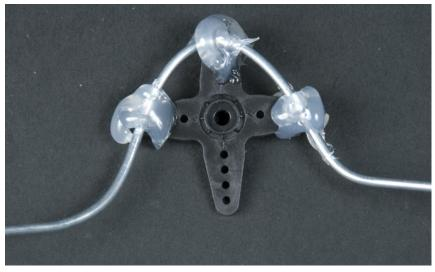
Figure 4-11. Securing with hot glue
