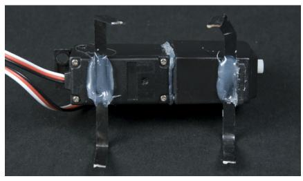
Figure 4-18. Gluing attachments
