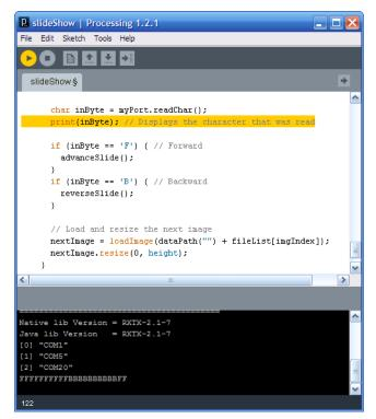
Figure 5-26. Processing displaying the characters it reads from the Arduino over the serial port
