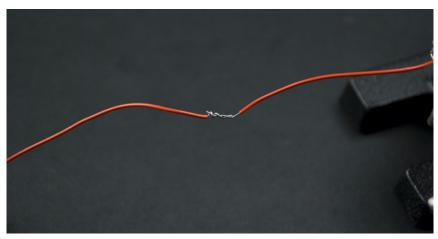
Figure 3-32. Wires with ends twisted together
