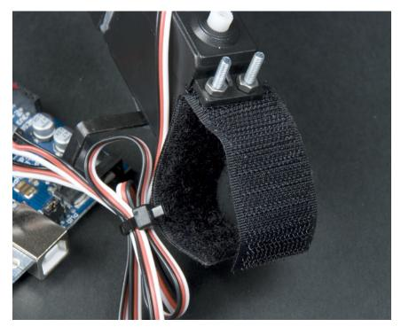
Figure 4-17. Velcro tape for the batteries
