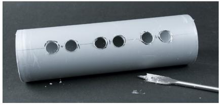
Figure 5-28. The 16mm holes for the sensors
