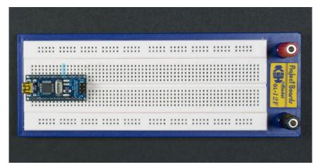
Figure 3-9. Arduino Nano on a breadboard
