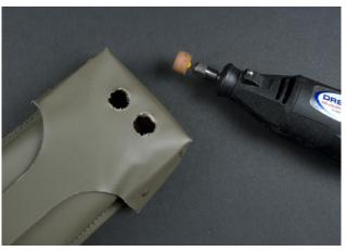
Figure 3-27. Holes created with a mini drill
