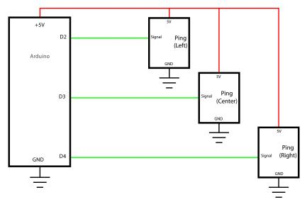
Figure 5-11. Connection diagram
