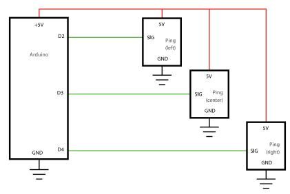
Figure 5-34. Connection diagram
