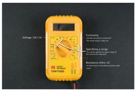
Figure 1-28. The most common functions of a multimeter
