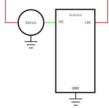
Figure 8-8. Connection diagram
