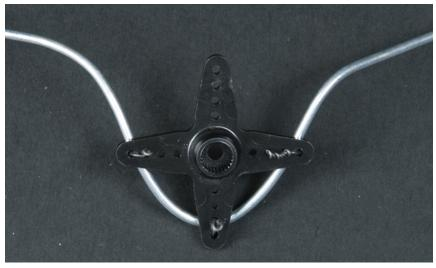
Figure 4-10. Attaching with metal wire
