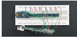
Figure 7-20. Six relays connected to control six buttons
