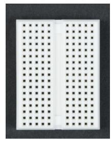
Figure 3-6. Small prototyping breadboard
