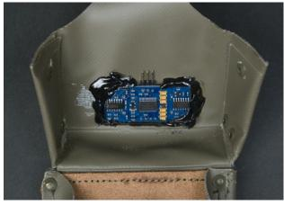
Figure 3-28. A hot-glued ultrasonic sensor
