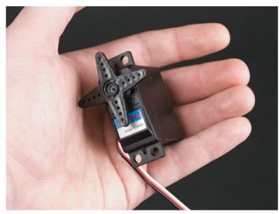
Figure 8-17. Finished continuous rotation servo
