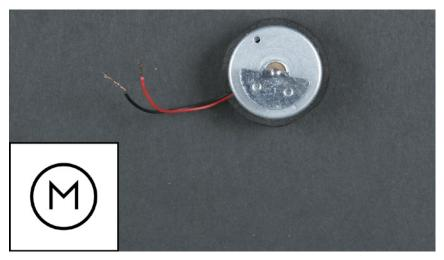
Figure 3-14. Vibration motor
