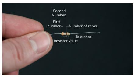
Figure 5-5. Reading a resistor's value
