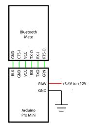
Figure 8-13. Arduino Pro Mini, Bluetooth Mate, and power supply connection diagram
