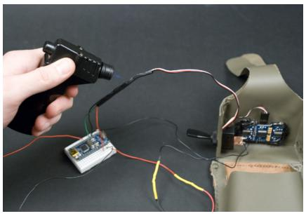
Figure 3-42. Attaching the heat-shrink tubing
