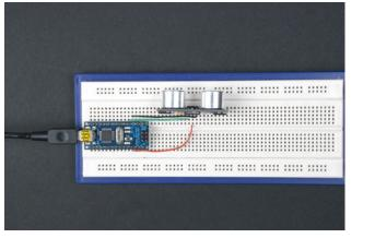
Figure 3-11. A connected ultrasonic sensor
