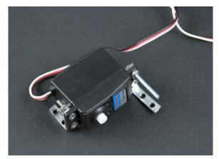
Figure 8-33. Kicker servo attachments from above
