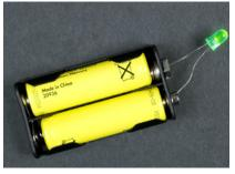
Figure 1-28. Simple closed circuit powering an LED
