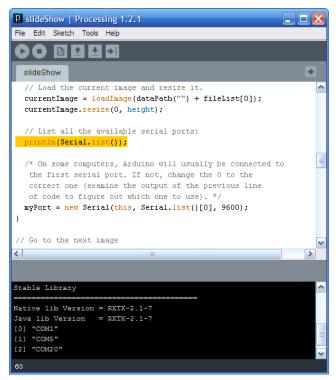
Figure 5-25. Processing listing its serial ports
