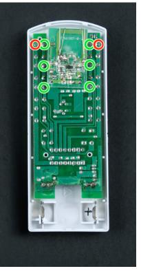
Figure 7-13. Solder pads: red wires to red ones and green wires to green ones
