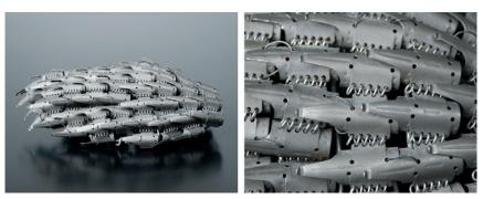
Figure 1-9. Porcupine robot cover made from a machine gun ammunition belt
