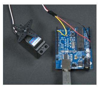
Figure 4-4. Servo connection
