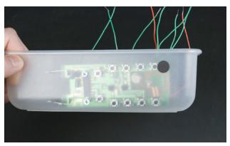
Figure 7-28. Circuit board attached, with a round sticker over the LED indicator light
