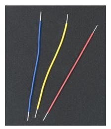
Figure 3-7. Jumper wires
