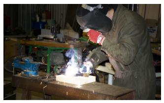
Figure 1-3. Welding a robot hand
