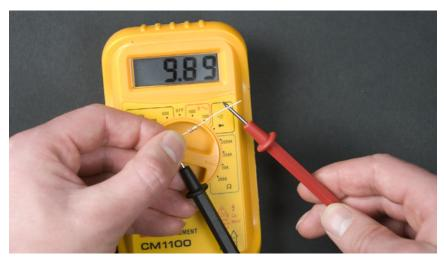
Figure 5-8. Measuring resistance with a multimeter
