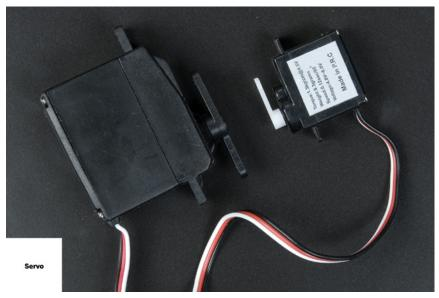
Figure 4-3. Two servo motors
