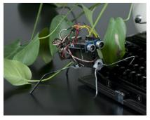
Figure 4-1. The completed Insect Robot
