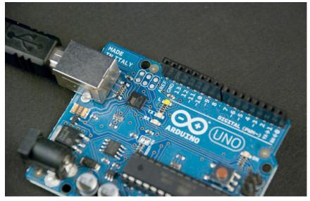
Figure 2-8. The LED on pin 13
