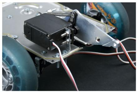
Figure 8-49. Kicking mechanism
