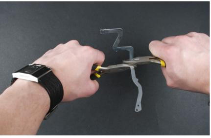
Figure 8-51. Cutting the front fork
