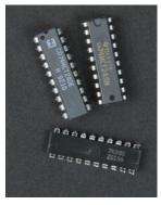
Figure 7-22. Integrated circuits
