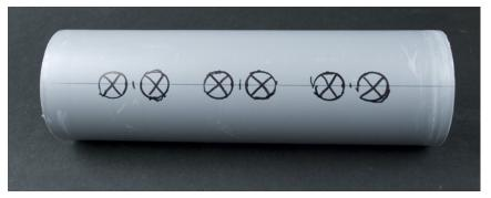
Figure 5-28. The marked ultrasonic sensor positions
