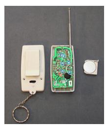
Figure 7-14. Solder pads on the Stanley wireless remote control
