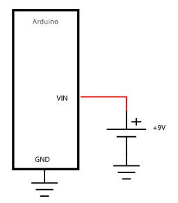
Figure 3-20. Arduino battery connection schematic
