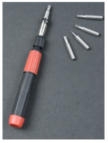
Figure 1-18. Screwdriver kit with a variety of bits
