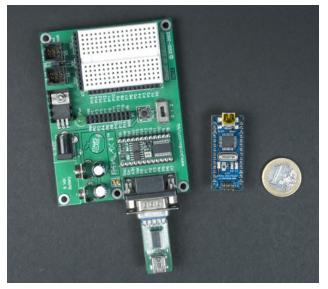
Figure 2-2. Basic Stamp (left) and Arduino Nano (right)
