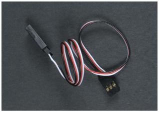
Figure 3-30. Servo extension cable
