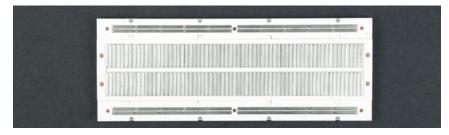
Figure 3-5. View of the bottom of the prototyping breadboard; metal plates conduct current from hole to hole
