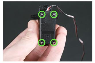
Figure 8-7. Screws to be removed
