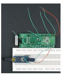
Figure 7-18. One relay controlling one button
