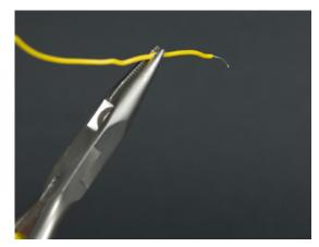
Figure 4-21. Bending the wire
