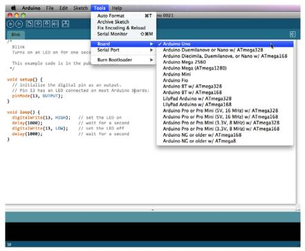
Figure 2-8. Arduino board selection
