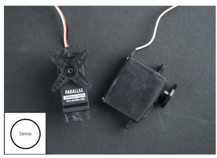
Figure 8-5. Continuous rotation servos
