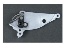
Figure 8-45. Kicker leg with servo horn attached
