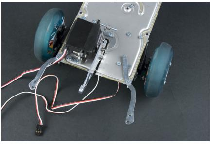
Figure 8-53. Front fork attached in place
