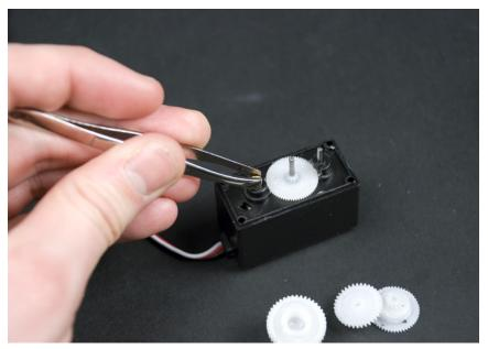
Figure 8-15. Adjusting the potentiometer to the center
