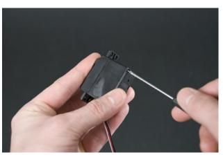
Figure 8-8. Loosening the screws
