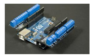
Figure 4-22. The ScrewShield
