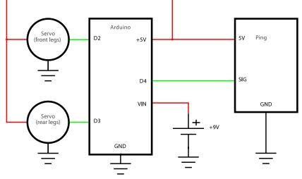
Figure 4-25. Ultrasonic sensor and servo connection schematic
