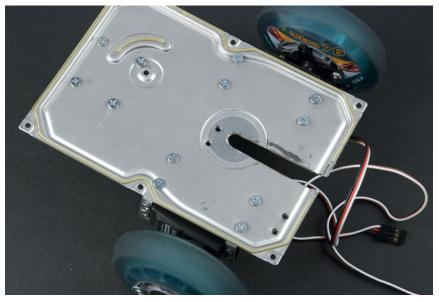
Figure 8-44. Front wheels attached
