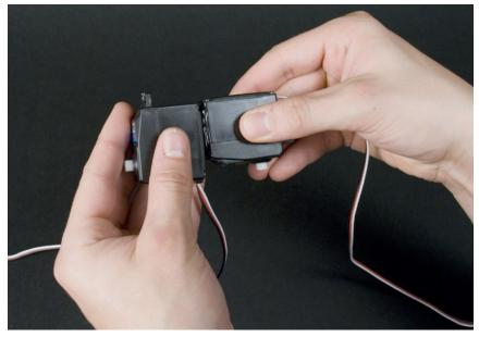
Figure 4-14. Gluing the servos together
