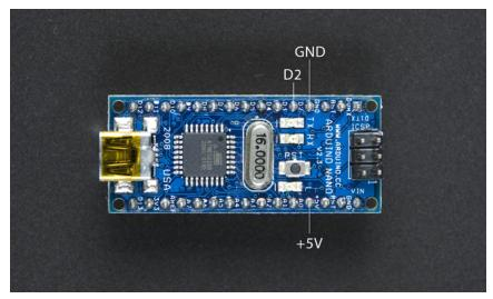
Figure 3-10. Arduino Nano pin assignments
