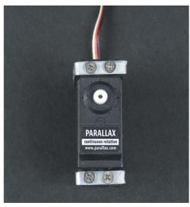
Figure 8-34. Wheel servo attachments from the front
