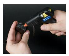
Figure 4-13. Spreading the hot glue
