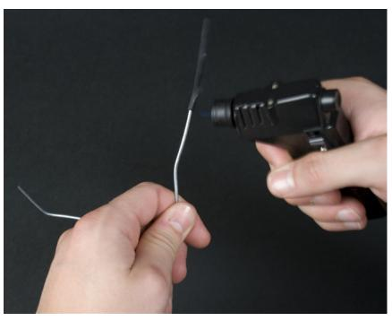
Figure 4-9. Attaching the heat-shrink tubing
