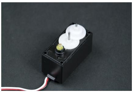
Figure 8-16. Using a drop of hot glue to hold the shaft of the potentiometer in place
