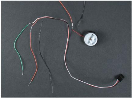
Figure 3-39. Single-strand wires soldered to the servo extension cable and to the vibration motor  $% \mathcal{A} = \mathcal{A} = \mathcal{A} + \mathcal{A}$
