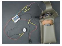
Figure 3-41. All components attached together; heat-shrink tubing covers the soldered points
