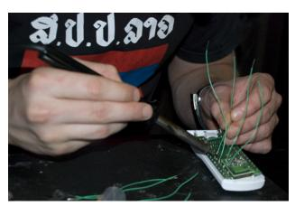
Figure 7-15. Soldering wires to the remote control switches
