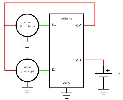
Figure 4-19. Servo connection schematic
