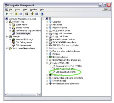
Figure 2-7. Determine the correct port
