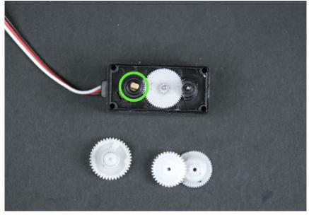
Figure 8-12. Shaft of the potentiometer
