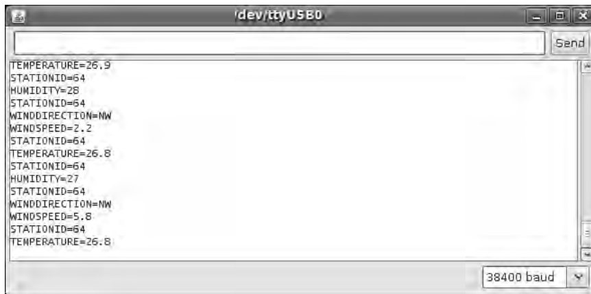
Figure 13-13. Weather Station Receiver values reported via the serial console
