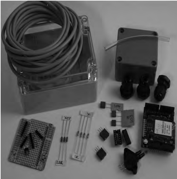
Figure 12-1. Parts required for water tank depth sensor
