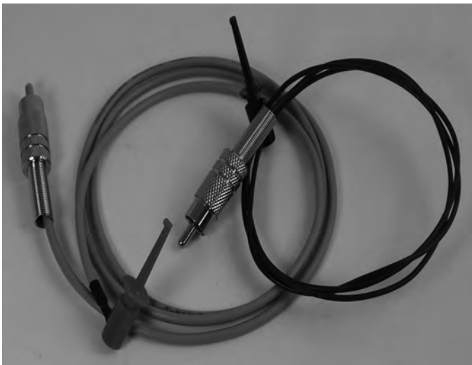
Figure 11-8. Ground probe and test probe
