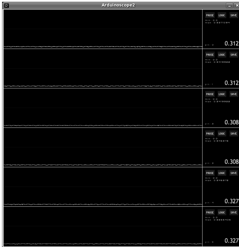
Figure 11-11. Arduinoscope program running on a host connected to an Arduino
