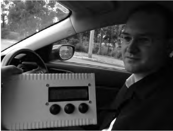
Figure 15-3. Arduino-based Vehicle Telemetry Platform
