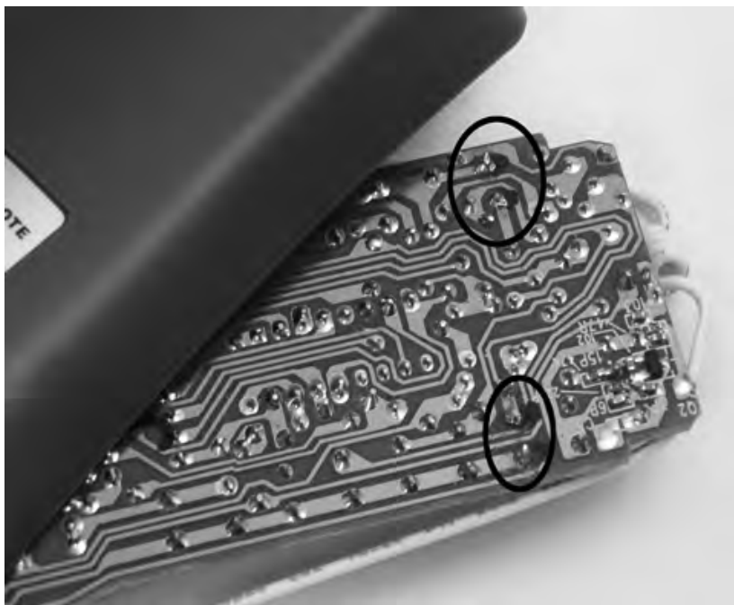
Figure 2-4. PCB of appliance remote control transmitter
