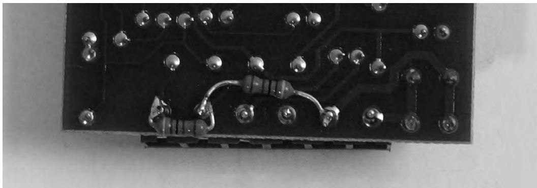
Figure 6-15. End-Of-Line resistors soldered in place on the PIR circuit board make installation much easier
