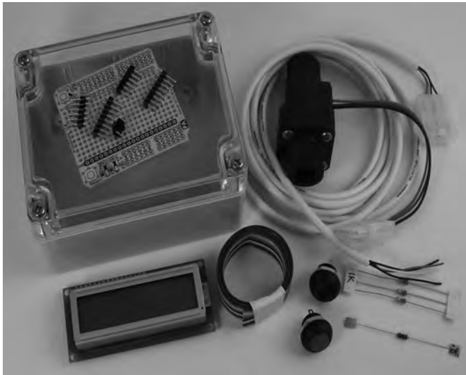
Figure 10-1. Parts required for water flow gauge
