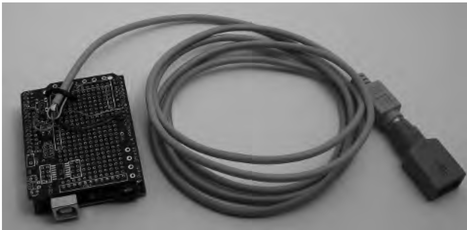
Figure 5-9. PS/2 extension cable attached to shield
