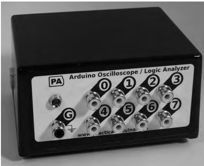
Figure 11-6. Connectors and LED mounted in front panel
