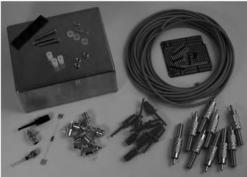
Figure 11-2. Parts required for Arduino Oscilloscope / Logic Analyzer
