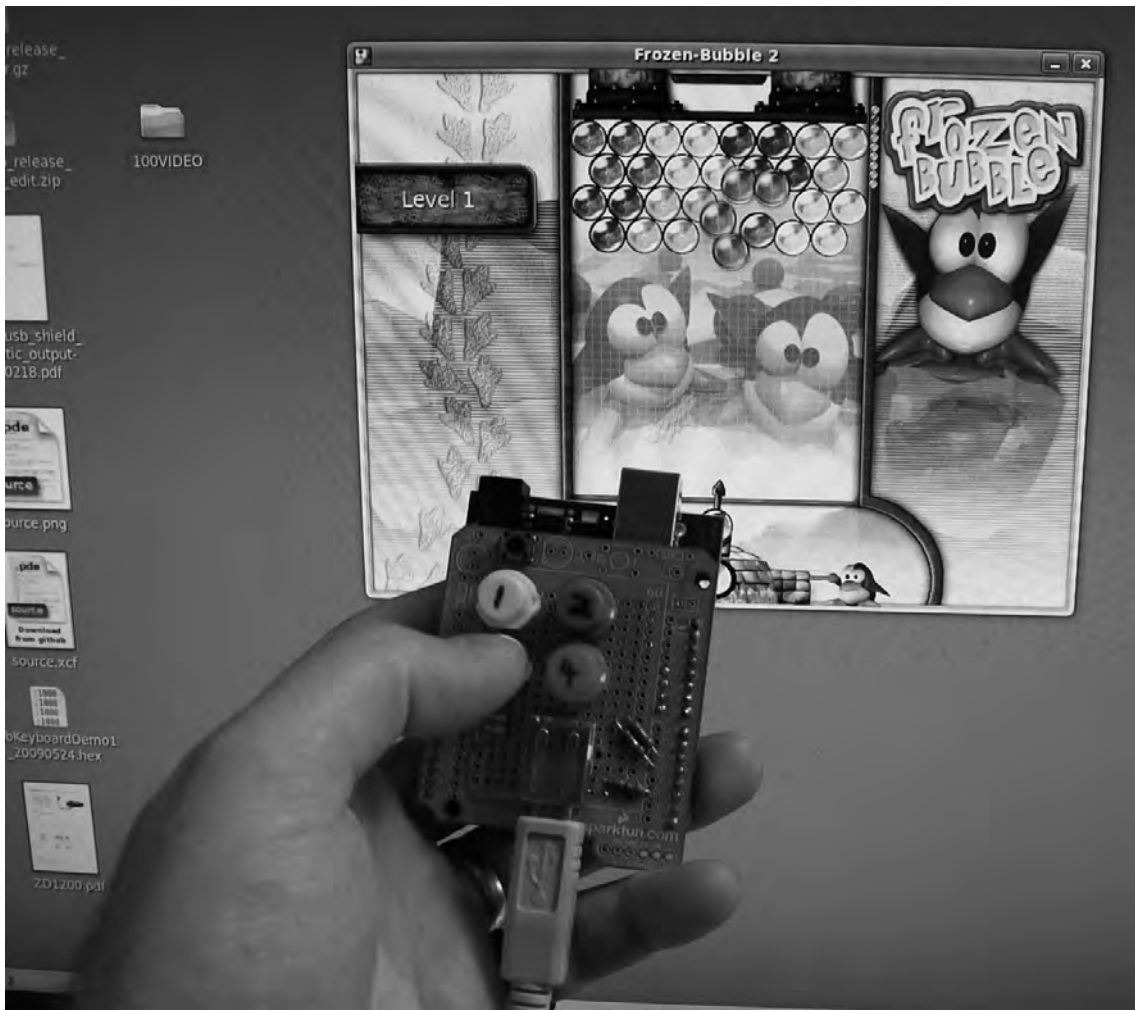
Figure 4-5. Using the virtual USB keyboard as a custom game controller
