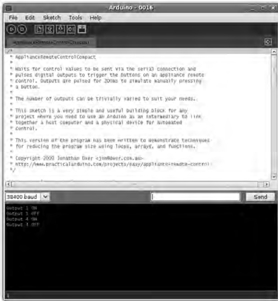
Figure 2-13. Serial monitor in Arduino IDE
