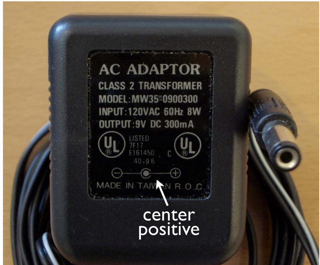
Actually input voltage can be from like 7.5V to 35V, but don't go over 15V so the voltage regulator doesn't have to work so hard.
