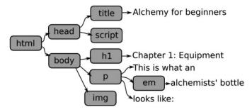
The document object model is based on such a view of the document. Note that the tree contains two types of elements: nodes, which are shown as boxes, and pieces of simple text. The pieces of text, as we will see, work somewhat differently than the other elements. For one thing, they never have children.
