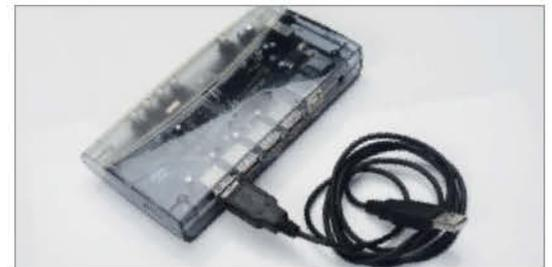
■ This is a powered USB hub. It is known as 'powered' because it has a power supply to provide power to connected devices
