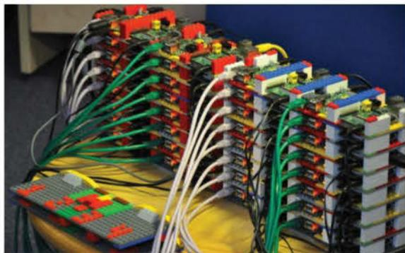
■ Lego features highly in the project, but so does research. Although the supercomputer uses an ordinary downloadable system image from the Raspberry Pi website, the performance and various other parts of the firmware and drivers have been improved by a factor of 50 or more.
