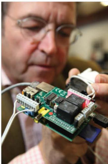
■ The hardware architecture was altered during the project so that it would work with mobiles (with Android and USB OTG) and desktop PCs too. It works with Raspberry Pi through SPI, but also through USB.
