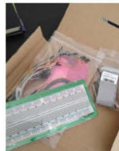
Extra electronics are needed on top of the Lego and the Raspberry Pi. The Cobbler breakout kit from Adafruit broke out the power, GPIO, I2C and SPI pins from the 26-pin header onto a solderless breadboard
