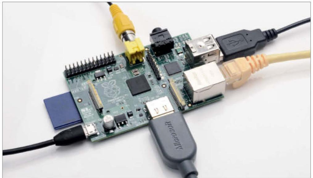
■ An operational Raspberry Pi - with USB, ethernet, HDMI, micro-USB and video out ports in use. One or more of these will be connected, depending on what you're using your Pi for. The Model B+ does not have a video out port
