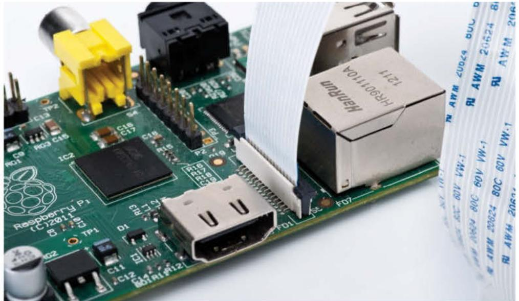
■ Fig 1. – Position the camera module's ribbon so that the silver side is facing the HDMI port
