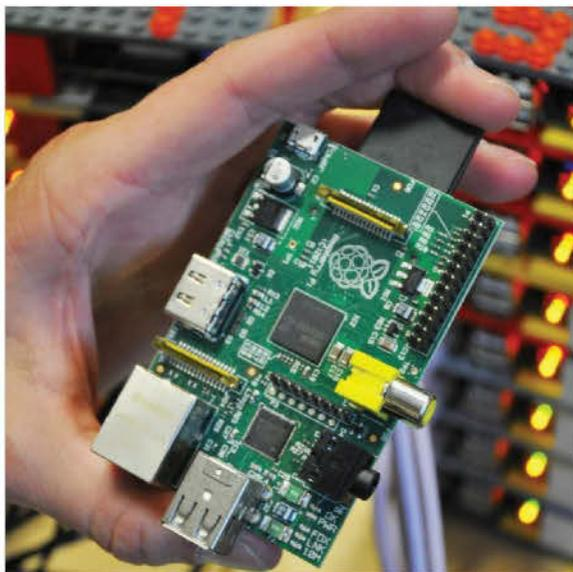
■ Since the drivers for the Pi’s video card are open source, the potential to use that video chip for processing opens up 24 gigaflops of general-purpose computer performance.
