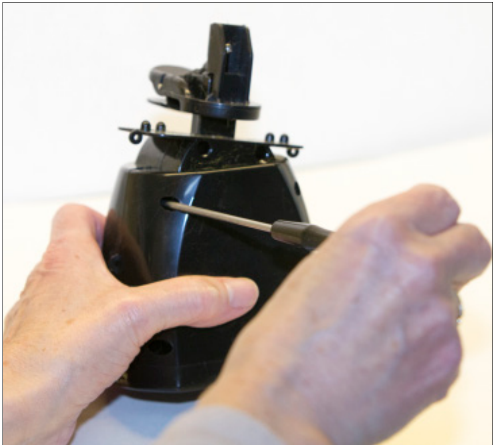
FIGURE 10-2: Removing the case of the movement mechanism.
