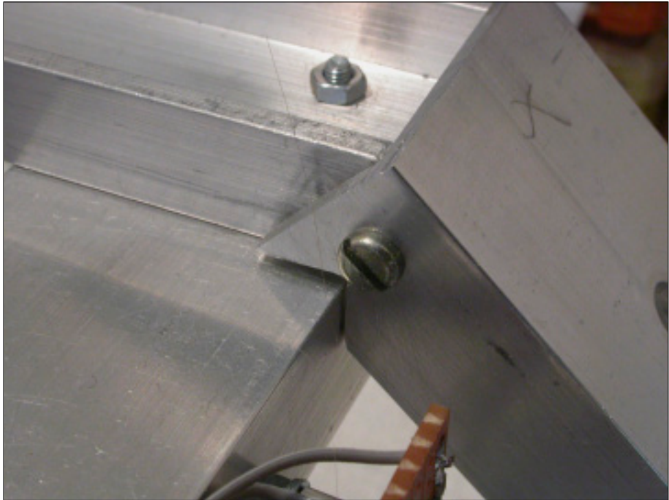
FIGURE 16-6: The notch needed on one side of each angled channel.
