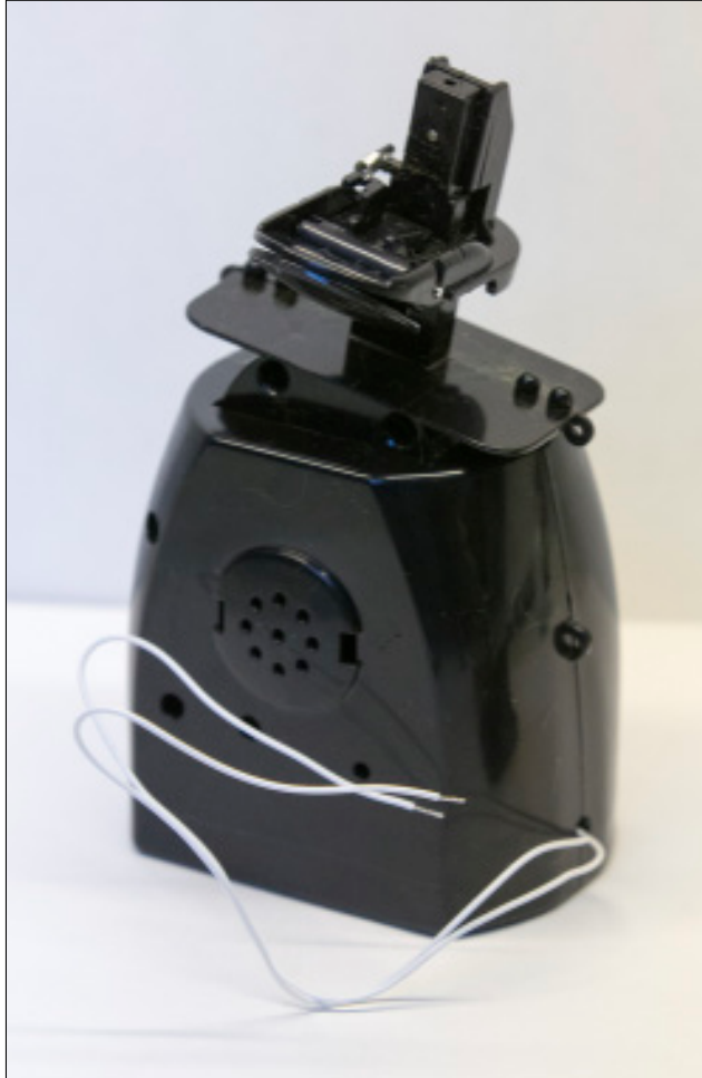
FIGURE 10-4: Toy post-surgery showing no ill effects. Touch the wires together to make the toy move.
