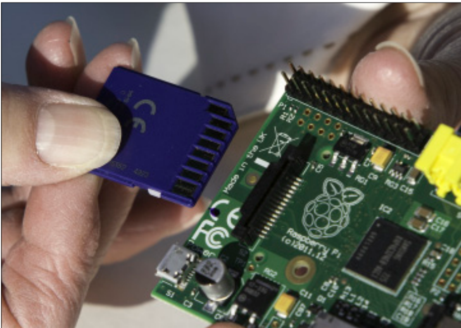
FIGURE 1-10: Insert the SD card carefully.
