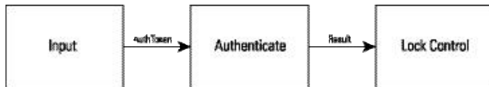
FIGURE 12-1: The system diagram of the door lock.
