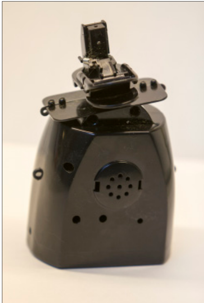
FIGURE 10-1: A naked chicken – the mechanism that makes the toy move.
