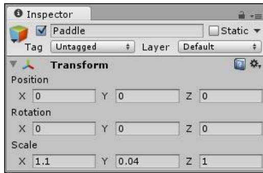
In the Unity environment, the **Transform** component of our **Paddle** was set to position **0** in the X-axis. But, we changed this with our line of code, setting the `x` property of the paddle's `transform` to `2`. The result is that the first time the `Update` function is called, the paddle appears to jump out of the way to two units along the X-axis.
